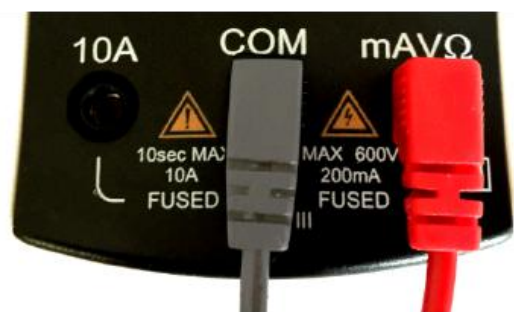
black probe in COM port red probe in mAVΩ port
